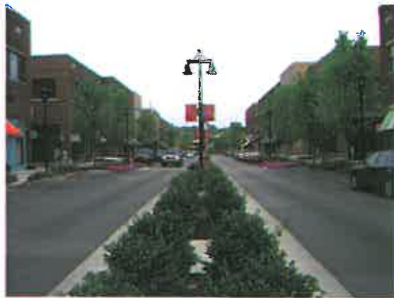
Refuge medians, special pavement treatments, narrow travel lanes, and on-street parking help to slow traffic speeds and create a bicycle and pedestrian-friendly environment.
